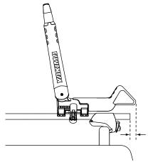
Position the tip of BowDown so that it protrudes slightly further than the crossbars.
