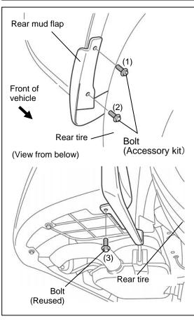
5. While pressing the rear mud flap against the rear bumper, install the bolts (2) included in the accessory kit and the reused bolt (1) in an order of (1) to (3) as shown in the figure.
