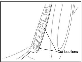
Pull back the splash shield and using nippers cut along the scribed lines on the underside in the cut locations shown in the figure.
