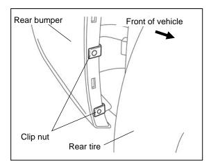
3. Install the clip nuts (2) to the rear bumper as shown in the figure and attach the splash shield.
