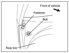
9. Install the rear mud flap to the rear bumper and reinstall the bolt (1) and fastener (1).
