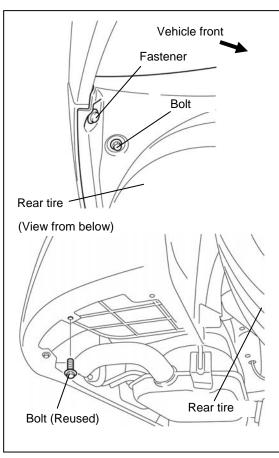
4. Install the bolt (2) and fastener (1).
