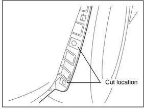
7. Pull back the splash shield and using nippers cut along the scribed lines on the underside in the cut locations shown in the figure.
