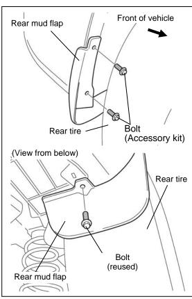
10. While pressing the rear mud flap against the rear bumper, install the bolts (2) included in the accessory kit and the reused bolts (1).
