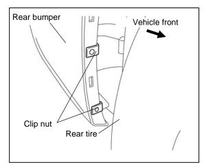
8. Install the clip nuts (2) to the rear bumper as shown in the figure and attach the splash shield.
