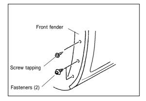
5-(1) Unscrew the screw tapping and fasteners.
