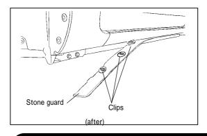
4-(4) Fit the clips (3) to the vehicle to place the stone guard (rear part) back into position.
