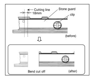
4-(3) Using a cutter knife or similar cutter, cut the stone guard at the position shown in the figure.
