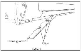
5-(4) Fit the clips (3) to the vehicle to place the stone guard (rear part) back into position.
