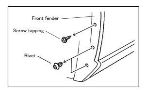
6-(1) Remove the screw tapping and two rivets.
