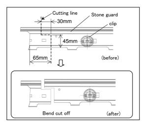
5-(3) Using a cutter knife or similar cutter, cut the stone guard at the position shown in the figure for vehicle which has the stone guard.
