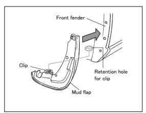
6-(2) Place the clip (bottom part of the flap) in the hole on the stone guard you removed at 5-(1) (Refer to the picture on the left). You will hear a clicking sound when it is installed correctly.
