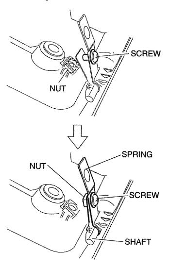
7. Install the screw and nut for the spring.
