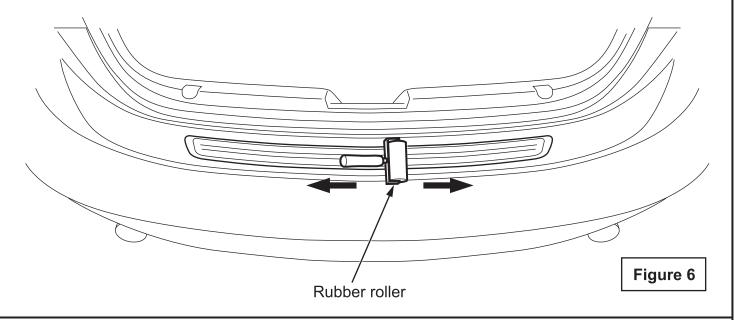
6. Inspect for proper adhesion and placement. Verify the part is not loose at any corner.
