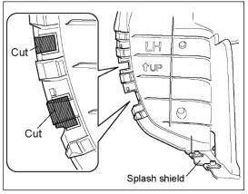
3. Use a nipper or similar to cut the splash shield along the notch lines on the underside of the splash shield. (2 place)
