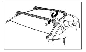
Shake the roof rack up, down and sideways to check that it is installed securely with no play or looseness.
