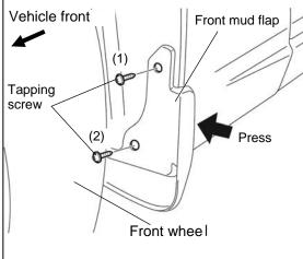
6. While pressing the front mud flap against the body, install the tapping screws in an order of (1) to (2) as shown in the figure.
