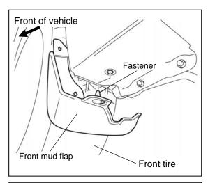
5. Install the fastener to the installation hole of the grommet removed in Procedure 1, and verify click sound.
