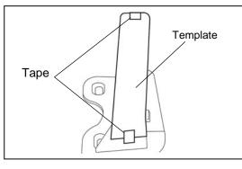
1. Align the template with the outer circumference of the accelerator pedal and attach.
