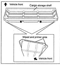
Make sure the installation surfaces of the Velcro (hard side), cushion tape on the ribbed underside of the cargo storage shelf are thoroughly wiped clean using a soft cloth dampened with isopropyl alcohol (IPA), and then apply primer.
