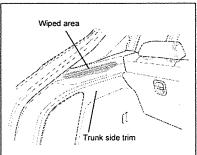
Make sure the installation surfaces of the velcro on the trunk side trim are thoroughly wiped clean using a soft cloth dampened with isopropyl alcohol (IPA).
