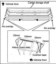
Peel off the backings of the Velcro (hard side) and the cushion tape, and affix them along edge line to the ribbed underside of the cargo storage shelf.
