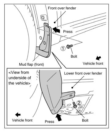
5. While pressing the mud flap (front) in the direction of the arrows shown in the figures, attach the bolts(2) in order from (A) to (B).
