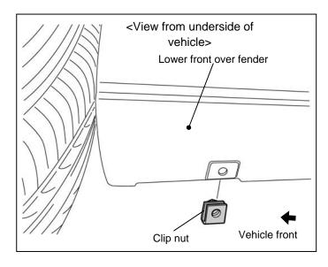
3. Align the lower front over fender underside hole, and install the clip nut (1).
