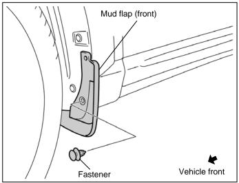
4. Align the mud flap (front) with the installation position and install the fastener (1).
