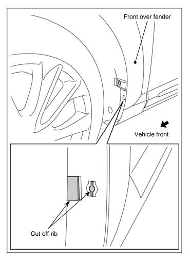
1. Cut off the ribs on the front over fender shown in the figure using nippers.
