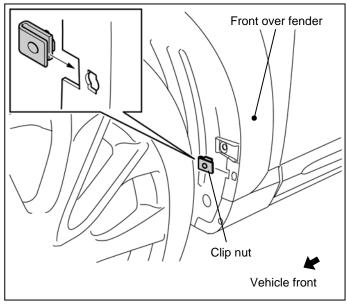
2 . Align the front over fender hole, and install the clip  $\operatorname{nut}$  (1).
