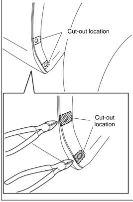
Cut using nippers in the cut-out locations along the scribed lines on the underside of the splash shield as shown in the figure.
