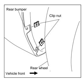
3. Install the clip nuts (2) to the rear bumper as shown in the figure.
