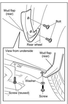
4. Install the mud flap (rear) to the rear bumper, and while pressing it against the rear bumper, install the screw (1), washer (1) and the bolts (2).
