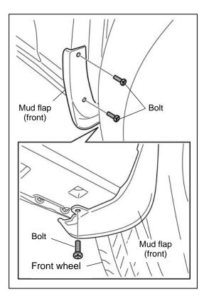
3. Install the mud flap (front) and the bolts (3).
