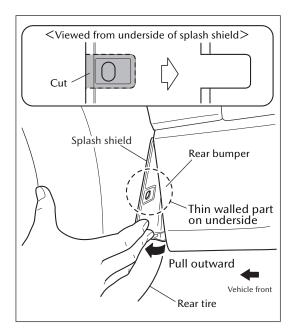
3. Use a nipper or similar to cut along the dotted part of the thin walled section on the underside of the splash shield.
