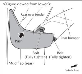
Install while pushing the mud flap (rear) in the direction of the arrow so that the gaps between the contact surfaces at the top and bottom of the V-groove are even.
