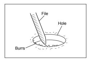
5. After drilling the hole, use a file to fully remove any burrs from the underside of the hole.
