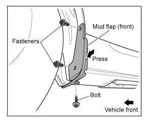
7. While pressing the mud flap (front) against the vehicle so that there are no gaps, install it by using the fasteners (2 places) and the bolt (1 place).
