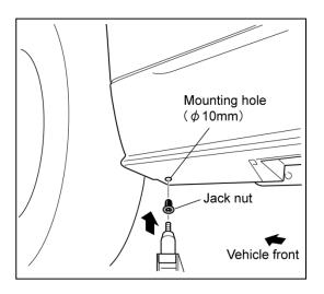
6. Insert the jack nut into the hole which was widened to a  $\phi$  10 mm, and then secure it using the jack nut tool.
