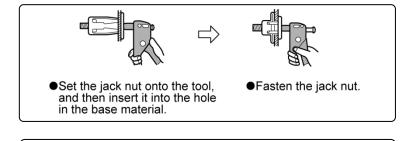
When securing the jack nut, be careful not to secure the mudguard at the same time.
