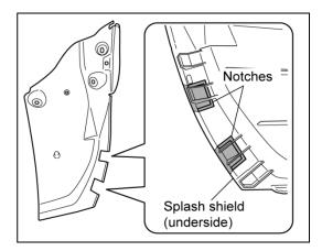
3. Use a nipper or similar to cut the splash shield along the notches on the underside of the splash shield. (2 places)
