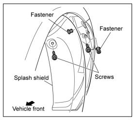
5. Install the splash shield with the fasteners (2 places) and the screws (2 places).
