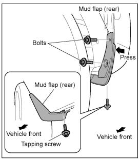
6. While pressing the mud flap (rear) against the vehicle so that there are no gaps, install it by using the bolts (2 places) and the tapping screw (1 place).
