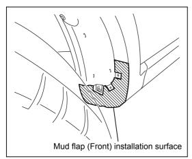
Use a soft cloth dampened with IPA (isopropyl alcohol) to clean the surface of the vehicle where the mud flap (front) is to be installed.
