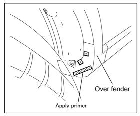
3. Apply primer to the double-sided adhesive tape adhesion surface of the mud flap for the over fender.
