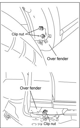
2. Align the over fender holes, and install the kit clip nuts (3).
