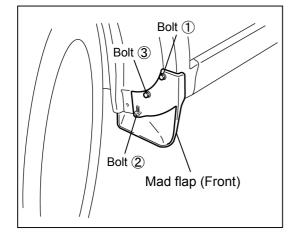
9. Install the mud flap (front) in the order shown in the figure on the left while pressing it against the over fender.
