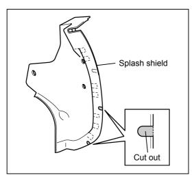
3. Cut off the splash shield shown in the figure using nipper (2 locations).
