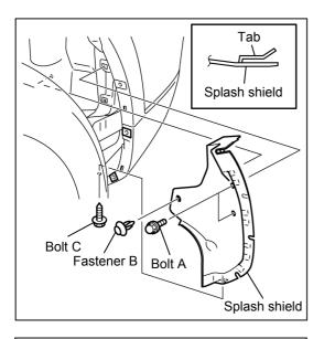
5. Place the splash shield back in its original position and install the bolt A (2), fastener B (1) and bolt C (1).
