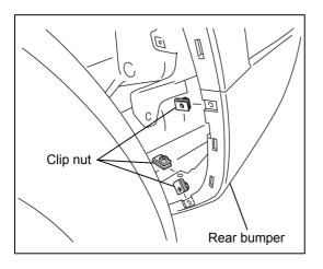
4. Align the rear bumper holes, and install the kit clip nuts (3).
