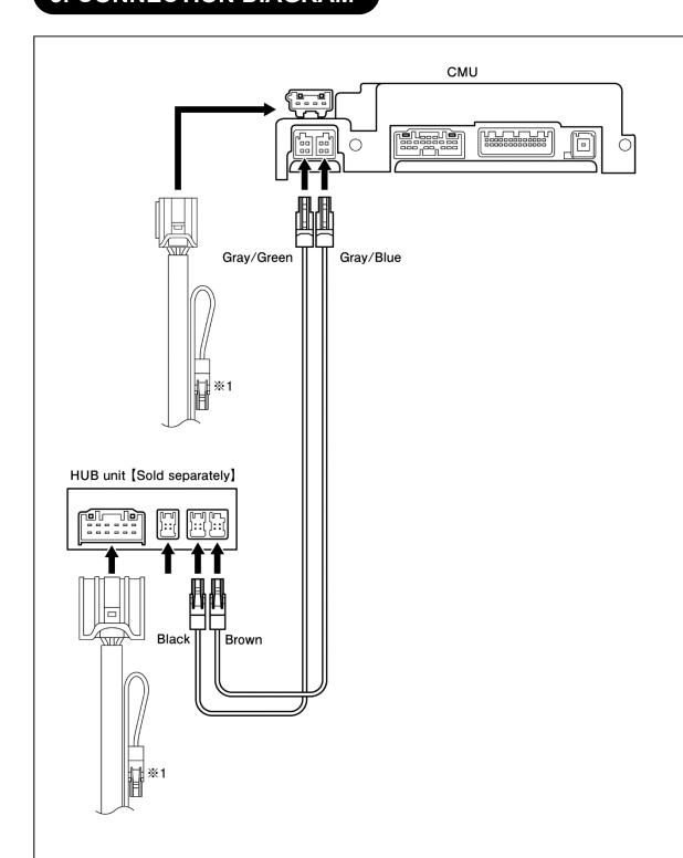
\*1: To prevent noise, wrap the disconnected vehicle wiring harness connector with a piece of sponge tape (100 x 30 mm).
